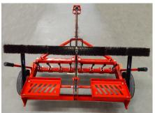
**Ballast Trays:** Two trays, each sized for standard cement blocks.
