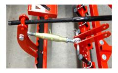
No Tools Required: Easily adjust cutting angle and depth without tools.
