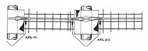
Now snap the remaining 18' ropes to the eyebolts at the side Velcro flap openings. Snap the ropes on the outside of the cage and run the cable under the net (or inside the cage) to the next arc. Weave it through the net and again snap the rope to the eyebolt outside the arc as you did in the above paragraph.
