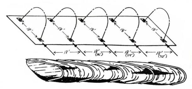
Each arch assembly will have a natural spread greater than 18'. Legs will have to be brought in to the 18' width.
