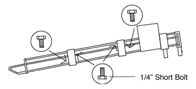
STEP 3: Place Washer Over Short Bolt. Screw on Nut And Tighten Nut (4X).
