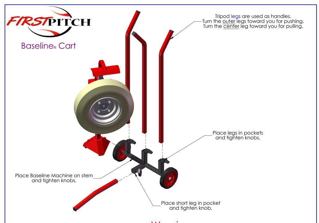
Warning: All knobs must be tightened before moving the machine around on the cart.
