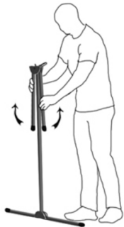
1. Place hinge on ground and swing open all four legs
