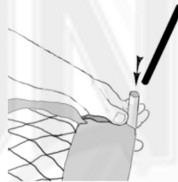
5. Slot pole (with groved top) into silver coupling of lower pole and slide orange sleeve up
