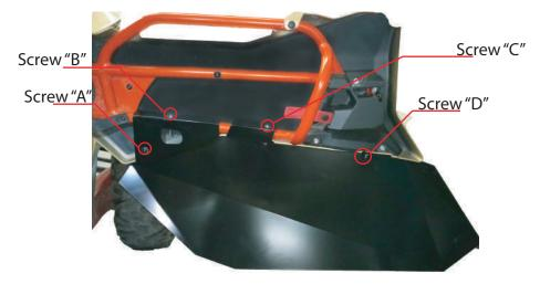
Adjust and hand tighten the "A" screw (original screw).
