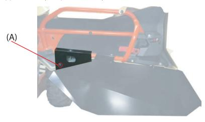
Remove the rivets from the handle guard on the inside of the door. Remove the handle guard and the plastic on the structure of the upper door.
