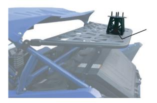
Place four chrome nuts on the spare tire carrier protruding bolts. As it is shown in the image
