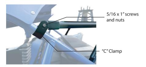
Place the "A" bracket in the lower part of the tubular of the vehicle, matching the perforations. Insert a 5/16 "x 1" bolt and nut facing down. As it is shown in the image.
