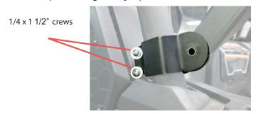
Place the bracket on the clamping arms (as it is shown in the image). Use one 3/8 x 1" screws with nut. (do not tighteen yet). Repeat step #1 and step #2 on the other side.
