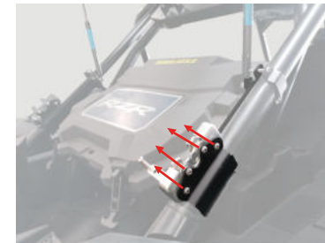
Direction of screws 1/4" x 1 1/2" toward indoors.
