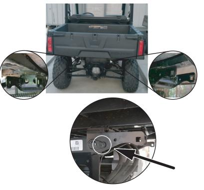
Place the hardware anchor on the vehicle depending the side. Put a spacer as shown in the picture below. Secure the anchor with a 3/8" x 3" Screw and lock nut, also put the screws of the vehicle (**Do not tighten yet**)
