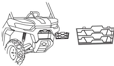
2 Remove the two bolts on the fornt of the vehice
