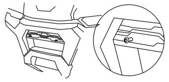
Place the bumper on the front of the vehicle. Align the mounting holes in the bumper to the holes ont the vehicle. Use (4x) 5/16" x 1" to secure the bumper.
