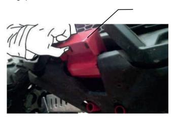
Mount the bumper above frontal support, align the perforations. (as it is shown in the image). Use two 1/4 x 2" screw with nuts and double washers.
