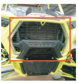
Locate the bumper starting from the central part. Use a two 3/8 x 3 1/2" screws with two flat washer, spacer and nuts (as it is shown in the image) (do not tighten yet).
