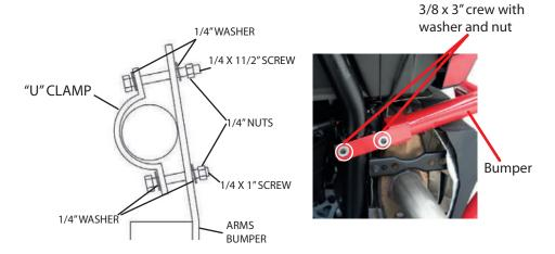
To finish the installation, tighten all the screws.
