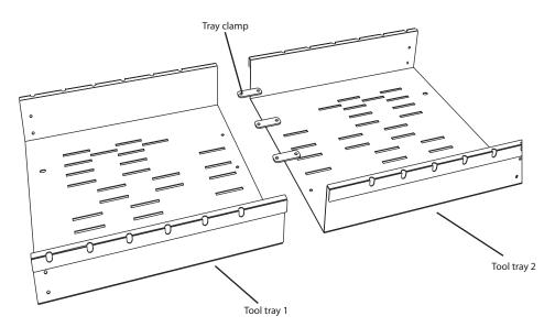
Assemble the Tool Tray. Use two 5/16" x 3/4" bolts and nuts on every side union.
