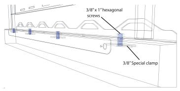
Make sure the hardware that secures the rear rack, aligns to the holes on the vehicle's bed. If not, change the position of the harware.
