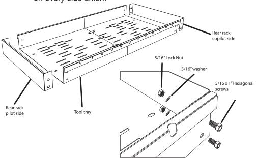
When the assembly of the Tool Tray is done, place it over both sides of the Rear Rack.
