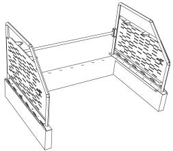
Insert the special clamps through the holes from the side Rear Rack and put the 3/8" x 1" hexagonal screw and washers up on the holes.
