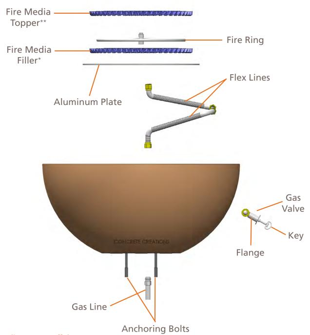
\* Install Gas line 1.5"- 2" off the center of the bowl, and 3.5"- 6" above ground level, subject to local codes.
