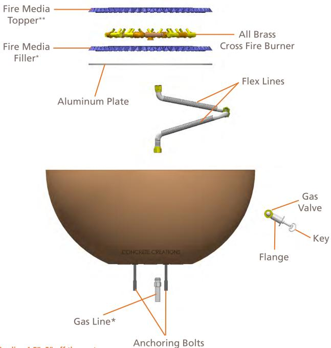
\* Install Gas line 1.5"- 2" off the center of the bowl, and 3.5"- 6" above ground level, subject to local codes.
