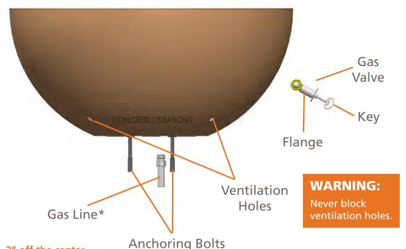
\* Install Gas line 1.5"- 2" off the center of the bowl, and 3.5"- 6" above ground level, subject to local codes.
