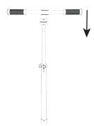
(1)Attach the horizontal rod to the handlebar fixed block
