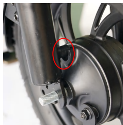
(5) Place the drum brake on the right side, align with the hole, and clamp down firmly
