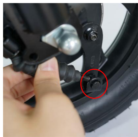
(12) Route the brake cable through the spring and sleeve
