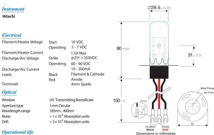
When radiant energy reaches 50% of the initial energy. Typical life 2000 hours Deuterium lamps are guaranteed for a period of one year from date of delivery or 2000 hours usage, which ever comes first.
