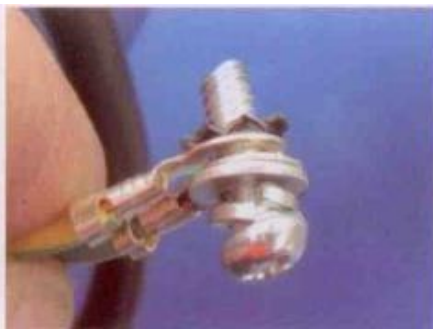
19. Screw the 2 Earth wires to the Saw Body as shown above. The correct assembly sequence is; Split Washer against head of Screw, Flat Washer, 2 Earth wires and lastly the Star Washer against the Saw Body. AN ELECTRICIAN WILL THEN BE ABLE TO TEST THE MACHINE IS EARTHED CORRECTLY. Plug the machine in and test the Stop Plate hits the Off Button just enough to switch off the machine without putting too much pressure on the switch. Adjust as necessary.
