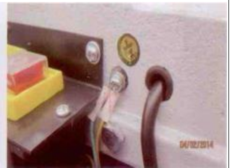
19. Screw the 2 Earth wires to the Saw Body as shown above. The correct assembly sequence is; Split Washer against head of Screw, Flat Washer, 2 Earth wires and lastly the Star Washer against the Saw Body. AN ELECTRICIAN WILL THEN BE ABLE TO TEST THE MACHINE IS EARTHED CORRECTLY. Plug the machine in and test the Stop Plate hits the Off Button just enough to switch off the machine without putting too much pressure on the switch. Adjust as necessary.
