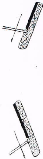
Pulling Weld Sloping downwards
