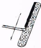
Pulling Weld Sloping upwards
