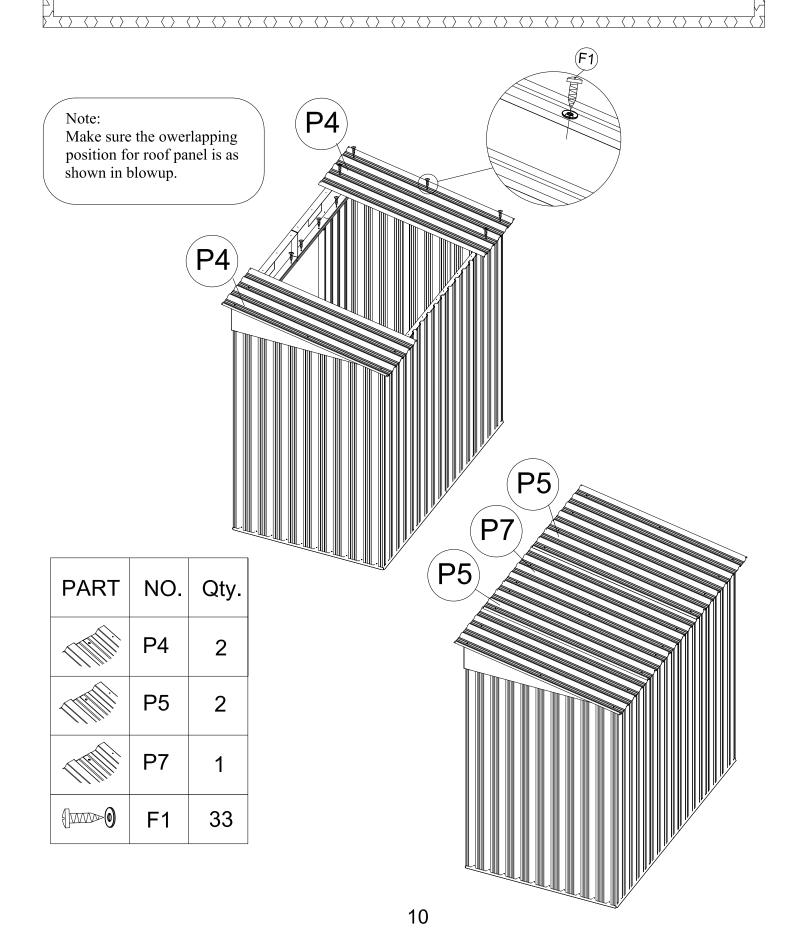
Assemble the roof flashing (15) and (17) with roof panels. Secure with (F1) screws with washers.
