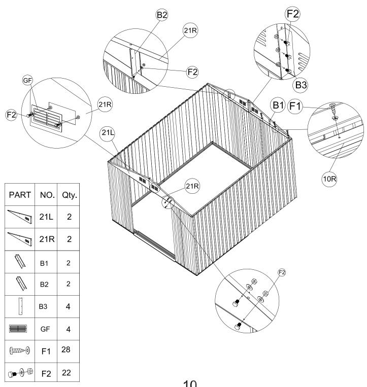
Join two roof supports (13) and (14) together, then fix 4 sets of roof stractures into the Gabel parels(21L) and (21R). Align the holes and secure with (F2) bolt and nut.
