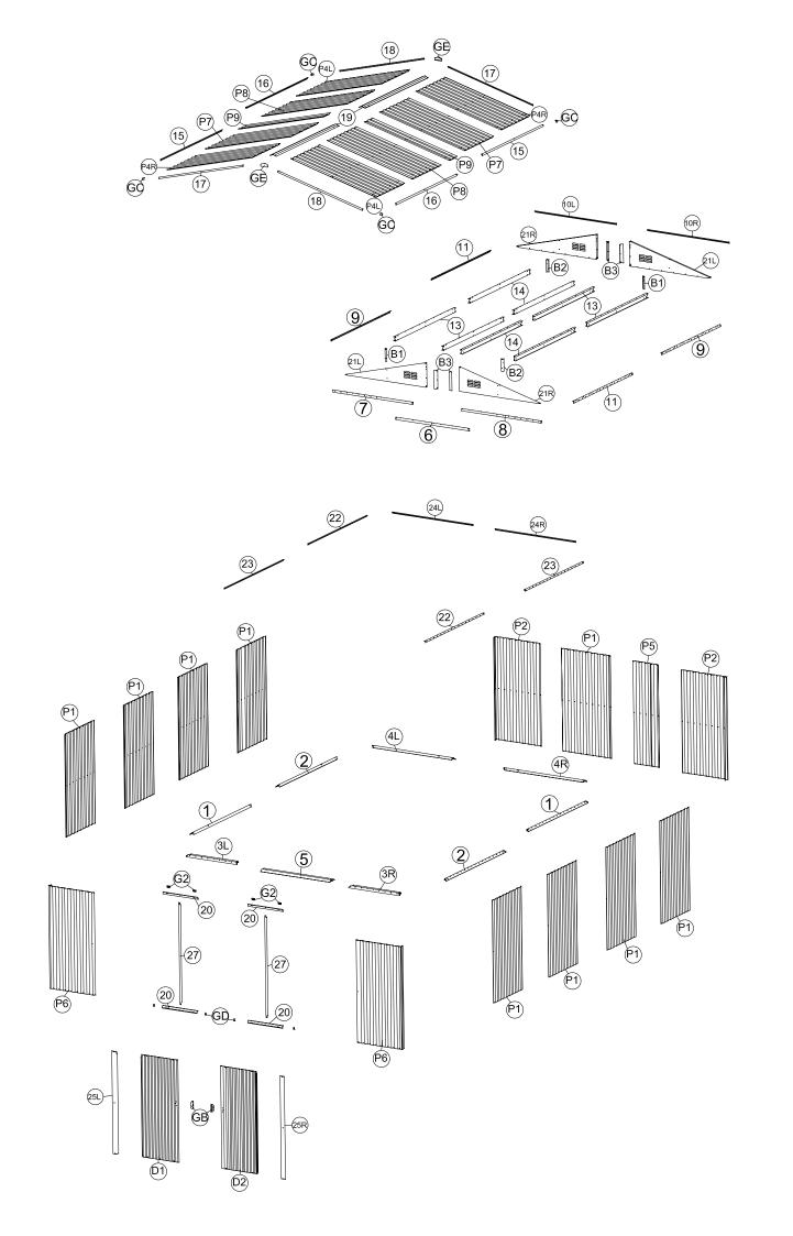
Assemble base bars from (2) to (4L) with (F1) screws. Then place the entrance taper channel (5) on top of the bar(3L) and(3R). Secure with (F1) screws to the foundation. Seeing the following figures .Make sure the base baassembly in a perfect square.
