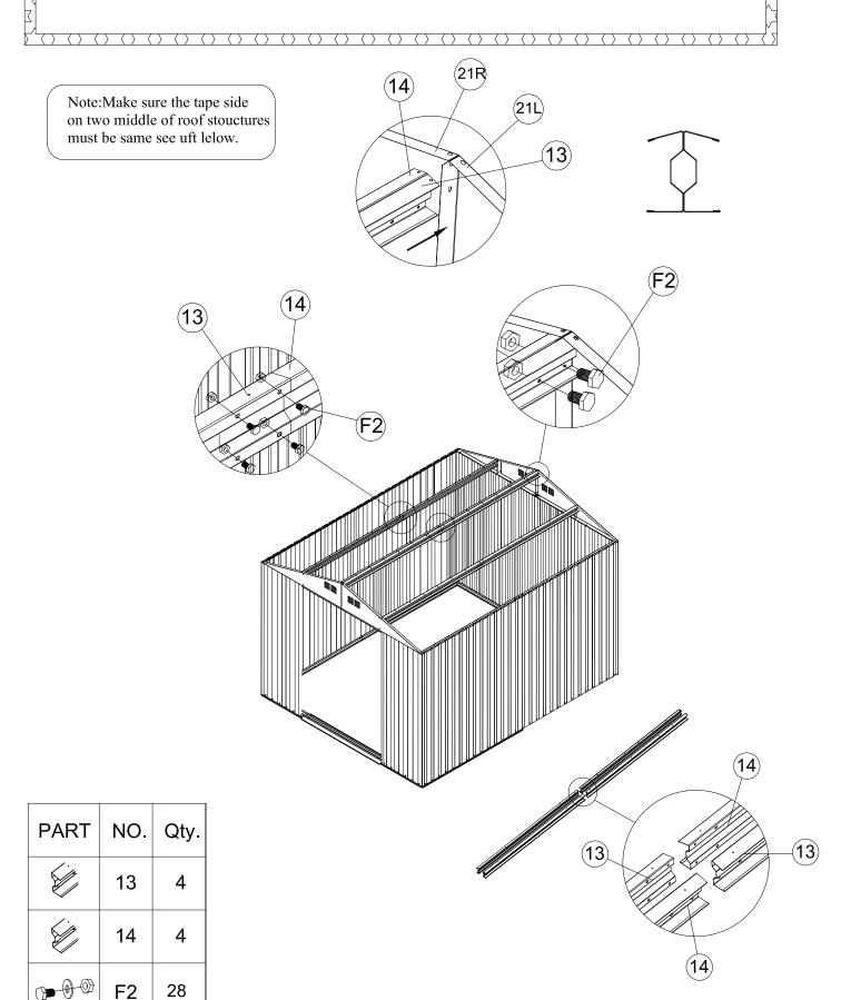
Place the roof panels (P4R) and(P4L) on the top of Gable panel (21L) and (21R). Line up the holes and secure with (F1) bolt, and nutwithwashers .Then place the roof panels (P7),(P8) and (P9) and secure them with (F1) screws with washers.
