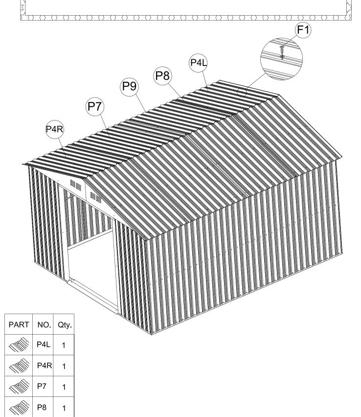
Assemble the roof flashing (15)(16), and (17),(18) with roof panels, secure with (F1) screws with washers. Then place 4 piece of top corner (GC) on the roof flashing joints. and secure with (F1) screws with washers.
