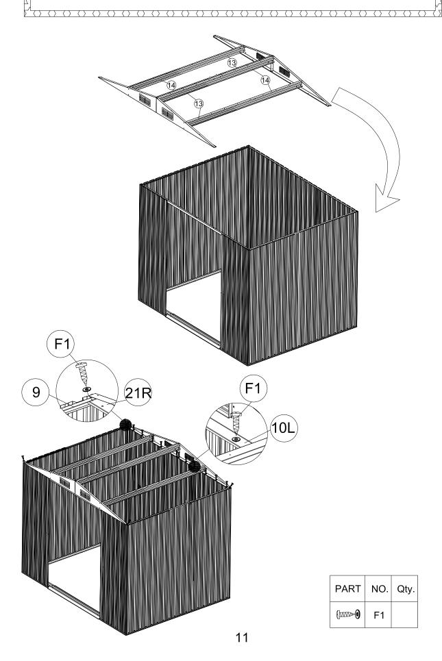
Place the roof panels (P5),(P6),(P8) and (P9) on the top of Gable panels and roof supports. Line up the boles and secure with (F1) bolt andnut with washers.
