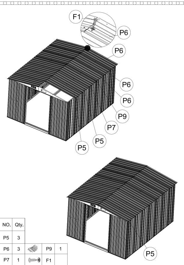
Assemble the roof flashing (15),(16) and (17),(18) with roof panels secure with (F1) screws with washers. Then place 4 piece of top corner (GC) on the roof flashing joints. and secure with (F1) screws with washers.
