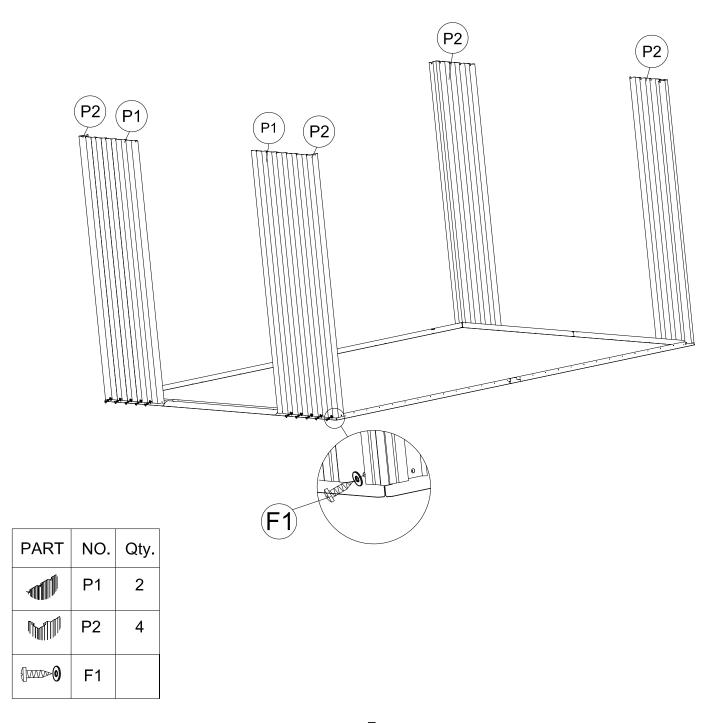
To assemble the strengthing bars (22),(23),(24L) and (24R) around the panels form inside as showed below. Secare them with (F1) screws with washers.
