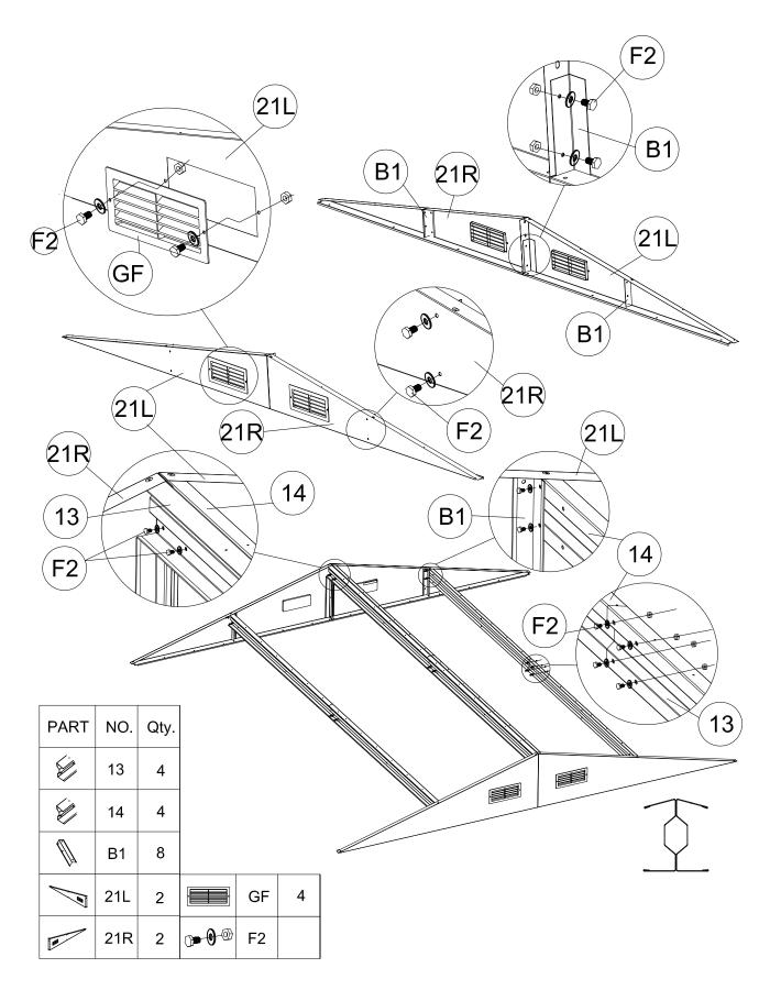
Place 4 piece of the Gable panels (21L) and (21R) (13) (14) on the top of the sliding channels (7).(8) and back top bars (10L).(10R), Align the holes and secure them with (F1) screws from inside as showed.
