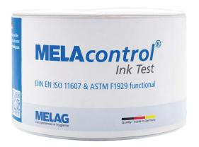
The ink required for the test comes in a practical disposable bag. The MELAcontrol Ink Test is sealed in a transparent sterilization package. Then the ink is pressed out. The spread of the ink tests all four sides of the packaging, revealing irregularities, flaws or channels in the seal seam.
