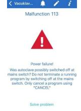
If the cycle malfunctions during operation, an alert with the malfunction number will be displayed. Along with the malfunction number, there will also be a description of the fault and step to take to troubleshoot the fault.
