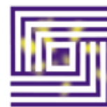
Fail - Wet steam
