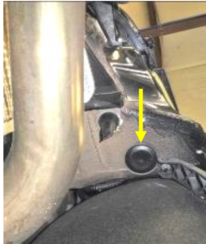
DRILL A 3/8" HOLE IN GROMMET
