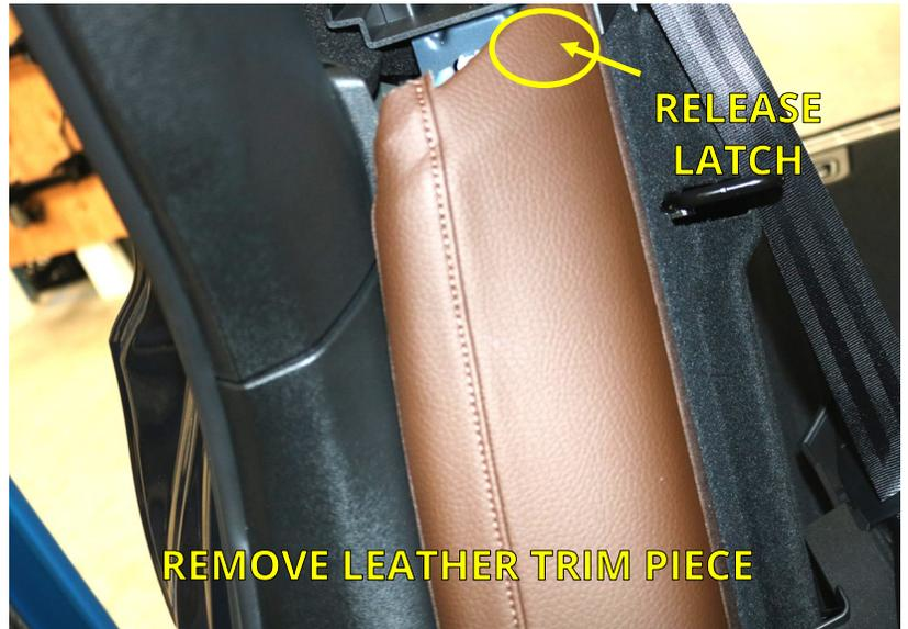
16. Pull inward to dislodge the passenger side panel. On the inside of the panel locate and disconnect the power plug and the light plug. Remove the panel.
