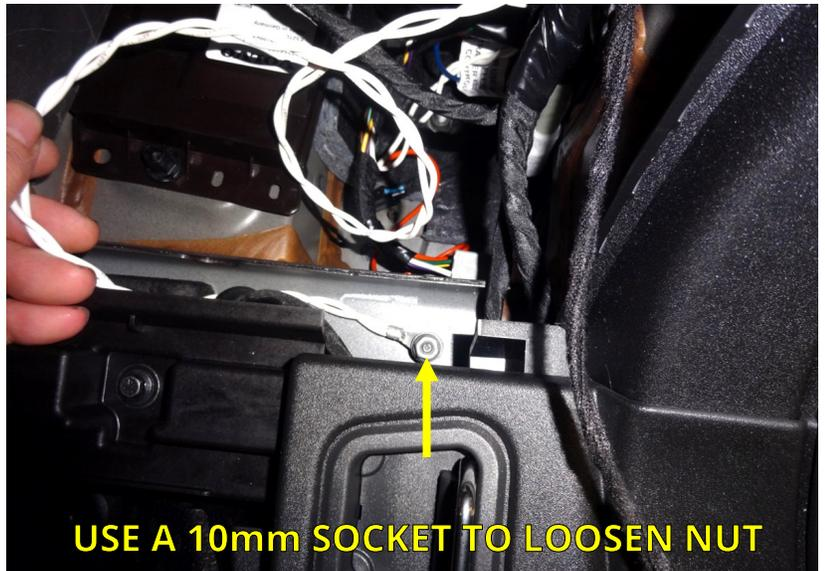
**USE A 10mm SOCKET TO LOOSEN NUT**
