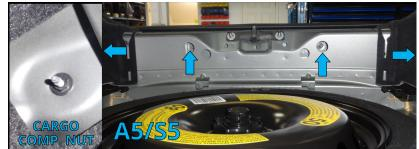
10. On both sides of the cargo compartment, remove the side rails by lifting up, as shown.
