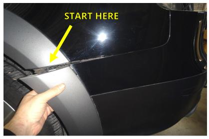
13. The fascia will not be completely disconnected from the vehicle, a wiring harness attached to the fascia must remain attached. Before removing the rear fascia, set up a stand or place a pad down near the rear of the vehicle. Carefully pull the fascia away from the vehicle and place on the stand or pad prepared earlier.
