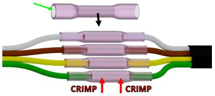
MATCH THE WIRE COLORS AND CRIMP EACH WIRE INTO THE SIDE OF EACH BUTT CONNECTOR. APPLY HEAT TO WATERPROOF AFTER CRIMPING
