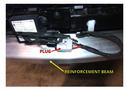
23. Remove the cap inside the plug by pushing the clip on top downward. Locate the power wire with plug located in the wiring kit. **Do not connect the plugs together at this time.**
