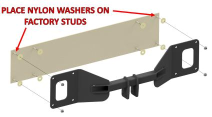
**USE 15mm SOCKET TO TIGHTEN OUTER NUTS**
