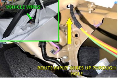
**NOTE:** Vehicles may have different wire colors than those shown. Verify circuits (wire colors) with multimeter.
