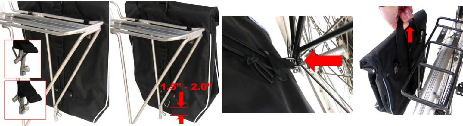
1. The pannier comes with an optional dropout hook, if you have a rack without an integral hook. Attach this dropout hook where the lower rack strut is attached to the bike frame.
