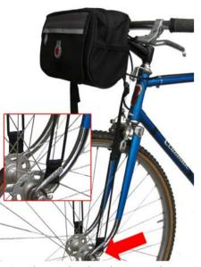
1. Attach the lower dropout hooks (included in the bag) on your fork's eyelets with bolts and nuts. Connect the elastic straps as shown and tighten the straps with the buckle.
