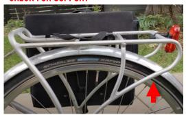
5. Not all racks are designed for panniers. Check your rack to make sure the pannier is supported from front to back. Pay attention to the rear edge. The best racks have a dog-leg type support (see arrow). We like the Axiom Journey. If heel clearance is an issue you may need and adjustable rack to move the pannier farther back. The chainstay length (too short) is a common root cause of heel strike issues
