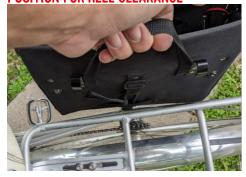
4. With the hook secure pull up on the handle and secure the upper hooks. Adjust the pannier forward or back as needed for heel clearance. The pannier
