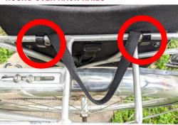
1. Start by resting the hooks over the rails. Hooks will fit rack tubing up to 16mm
