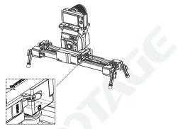
Step 3:Set up fully loaded slider at the angle you wish to use it and carefully test out counterweight. Increase or reduce weight accordingly. The pulley must be installed using an appropriate counterweight for the set up and weight of the camera and head.
