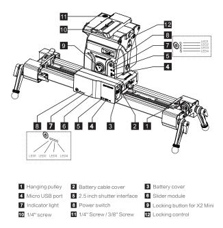
\*Micro USB port supplies power to Pan and Tilt Head and Slider or can be used to charge battery.
