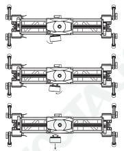
Firmly hold the flywheel and gently pull to the left, then do the same, but to the right followed by pulling the flywheel away from the carriage at 90 degrees. This will ensure safe removal of the flywheel from the carriage.
