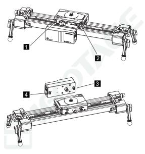
Step 3:Check that the single-axis module is securely attached to the carriage. Step 4:Check track is clear of obstruction. Step 5:install battery and switch on unit.
