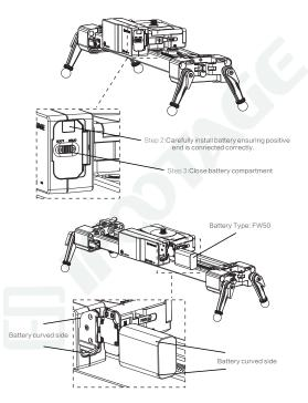
\*Insert the battery in the 1 - axis module, pay attention to the direction, DO NOT insert it in opposite direction.
