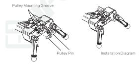
\*The carriage and camera may slip if the rake or slider set up angle is too steep. This can be prevented by using the pulley and correct counterweight. These should be removed when not in use.
