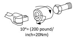
Tighten screw until the washer no longer rotates. Then tighten screw another 10° in same direction.
