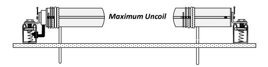
Adjustment is only possible with the DeadMan switch OFF, and after a motor limit has been reached or lift is stopped manually (white LED lights on controller are lit and stay on).
