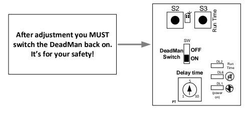
**DeadMan Function:** You use only the UP and DOWN buttons. You have to hold the button to make the lift move. When you release the button the equipment will stop immediately. If a key gets jammed you can stop the equipment with the stop button.
