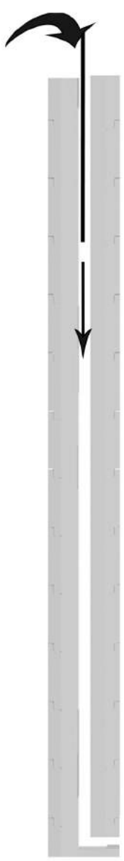
1. Push down wires from precut holes on ceiling
