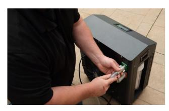
Screw the chiller hoses onto the inlet and outlet connections, Ensure they are tight.
