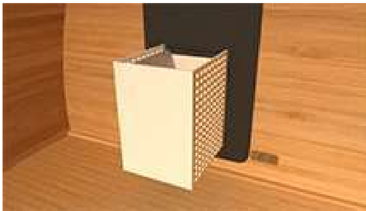
Inlet beside wood heater on Back wall
