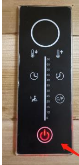
Sauna's Control Panel is OFF (power button is red)
