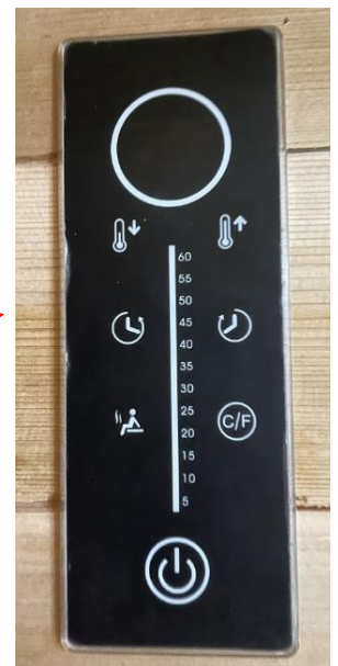
Sauna Control Panel has no Illumination
