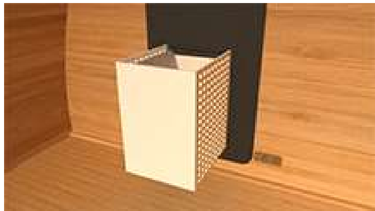
Inlet beside wood heater on Back wall
