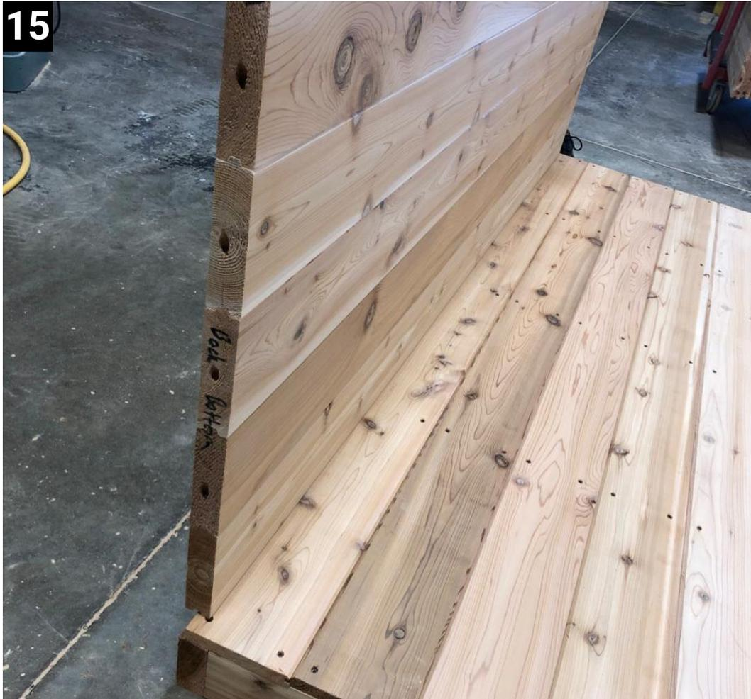
15 Start with the back bottom piece. Hold upright to help put the side pieces on.
