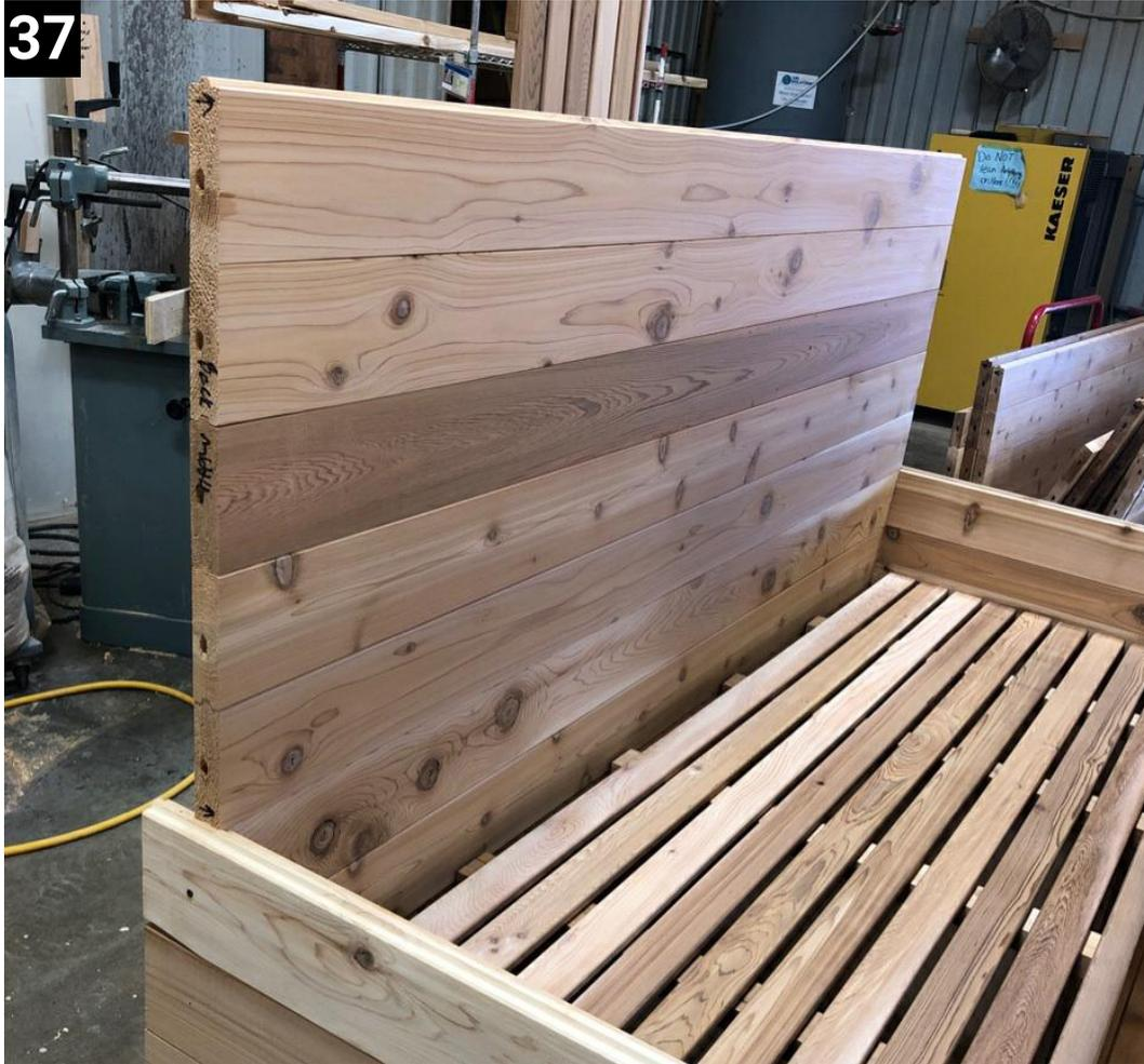
Attach the back middle piece to the bottom with 4" screws.
