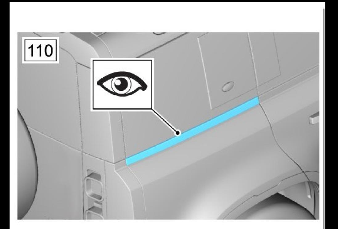
Mark the ditch finisher as shown and a drill a  $\frac{3}{4}$ " hole in both locations.
