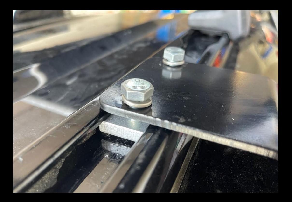
Install the black in spacers in to the  $\frac{3}{4}$ " holes as shown in sliver.
