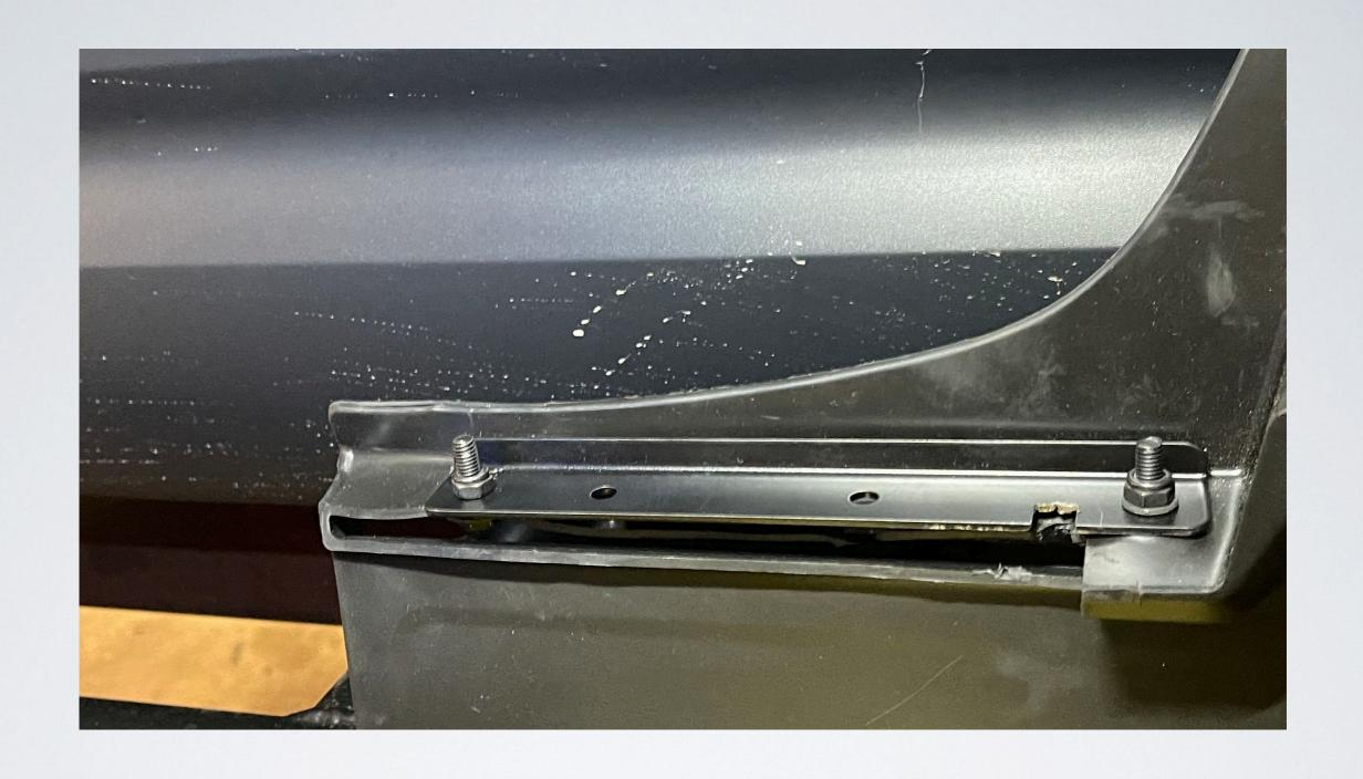
Place nut and bolt on the 2 ends of the sport bracket.
