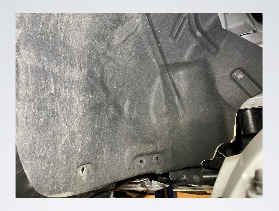
Pull the inner fender liner out
