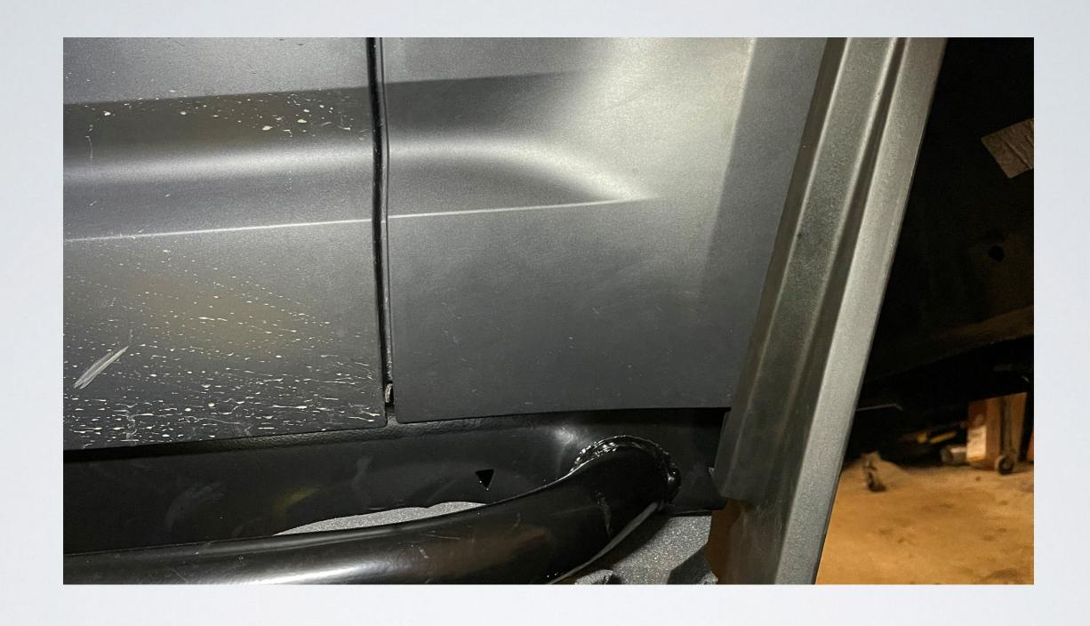
Test fit to make sure there is not interference with the slider.
