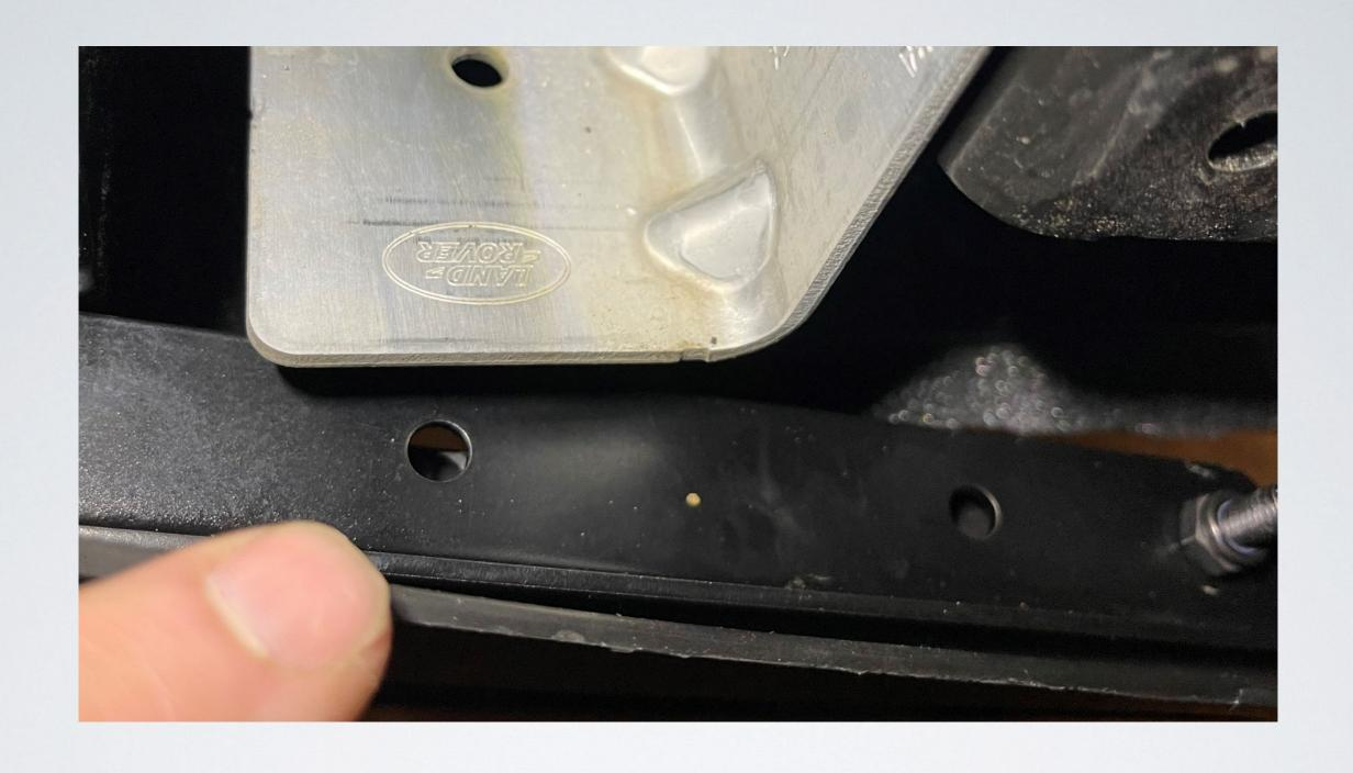
This hole needs to be aligned under the bracket with the Rover logo.
