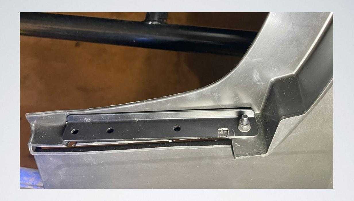
Notch the sport bracket so it will not interfere with the slider.
