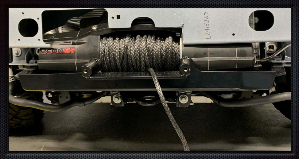
When everything is a-lined tighten the four winch mounting bolts to 45nm and the two lower winch tray brackets that mount to the factory recovery hook to 110nm
