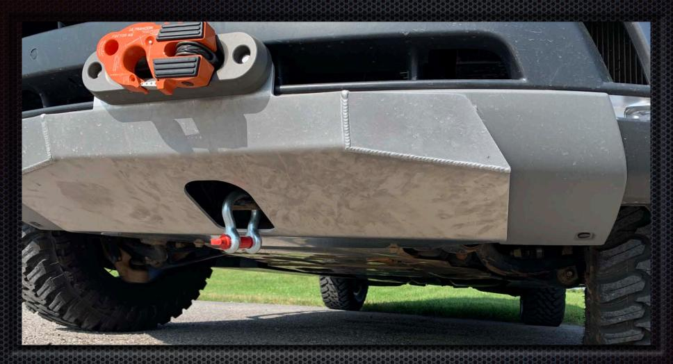
With everything in place tighten the four mounting bolts to 60nm
