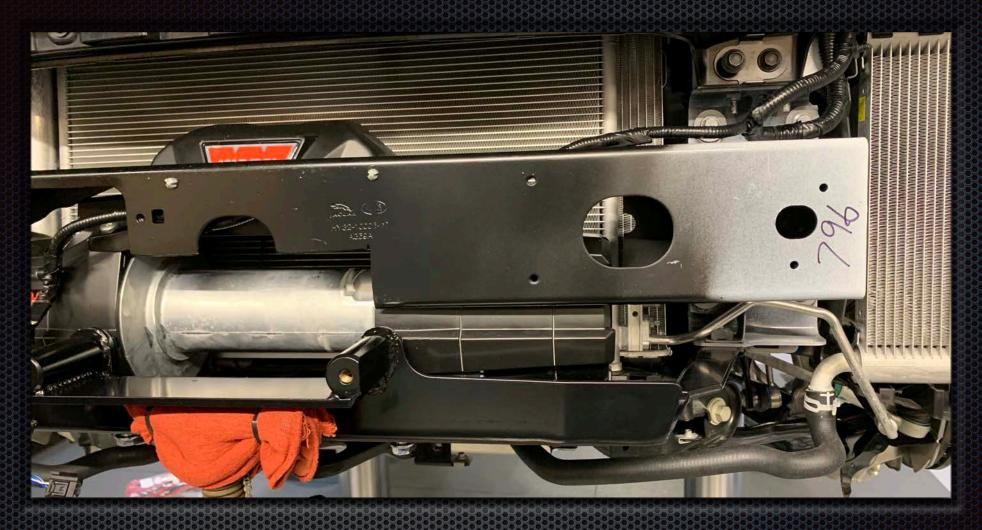
Install modified front bumper core support. Leaving out two upper inner mounting bolts. Tighten core support bolts to 55nm
