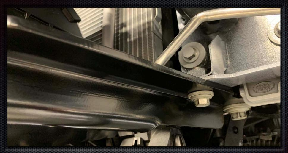
Install front winch tray bolts to front bumper core support and tighten to 100nm
