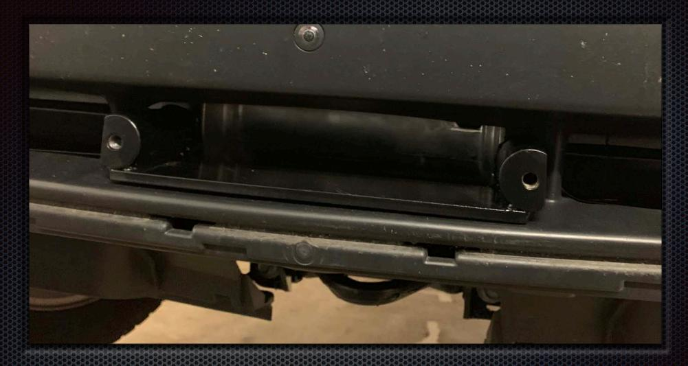
Slide the front bumper cover back on and a-line the winch tray to the center hole in the bumper cover. Reinstall the front bumper cover.
