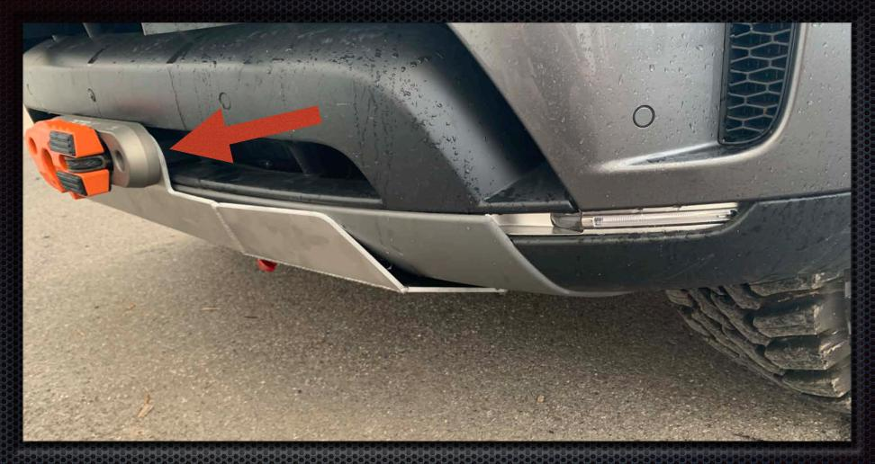
Loosely sandwich the fairlead and bash plates two upper mounting points to the winch tray.
