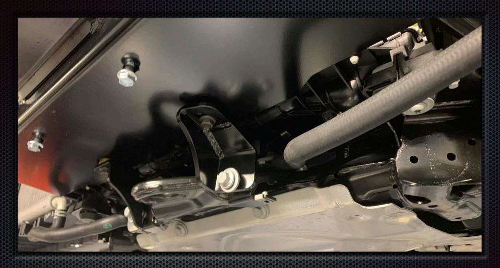
Loosely position the lower winch tray brackets to a-line with the winch mounting points and the factory recovery hook bolt holes.
