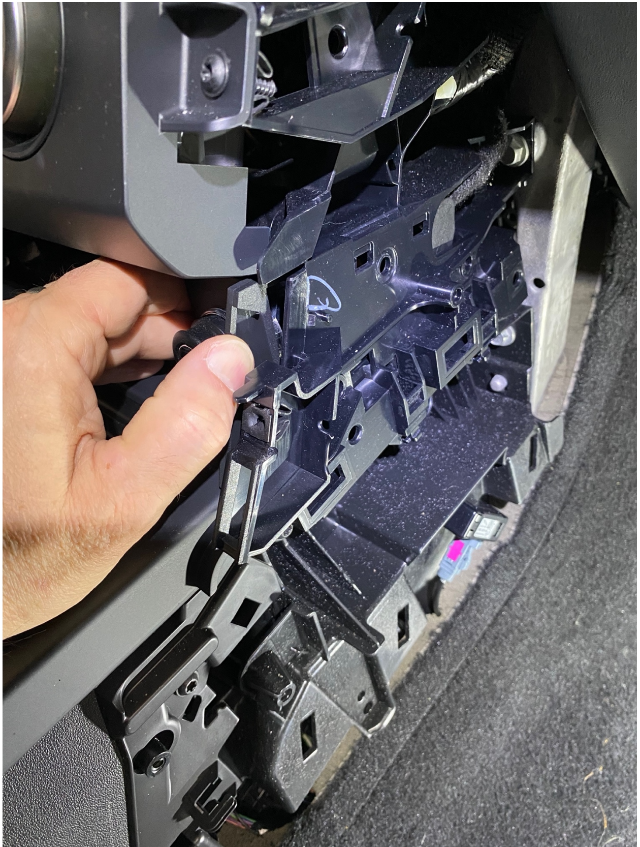
Once the screws are removed gently pull the cigarette lighter housing forward to remove
