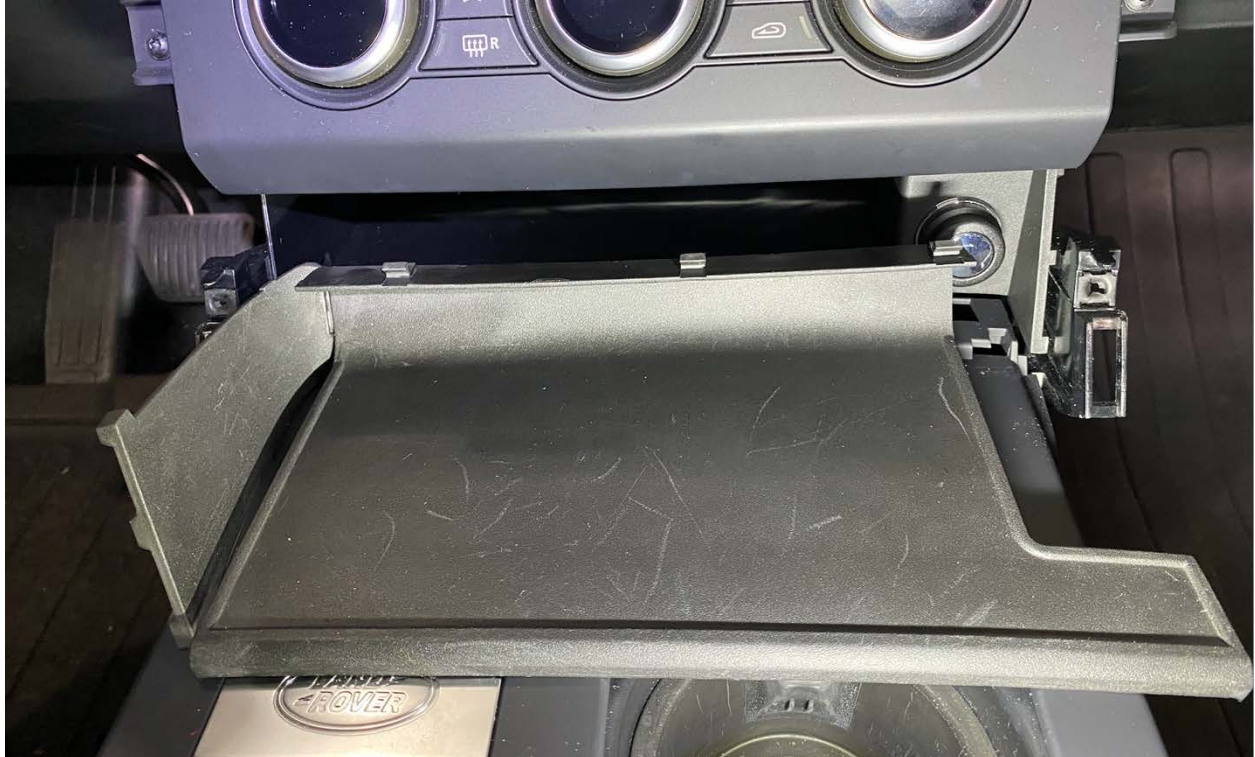
Slowly pull the rubber insert out and set aside (it will not be reused)
