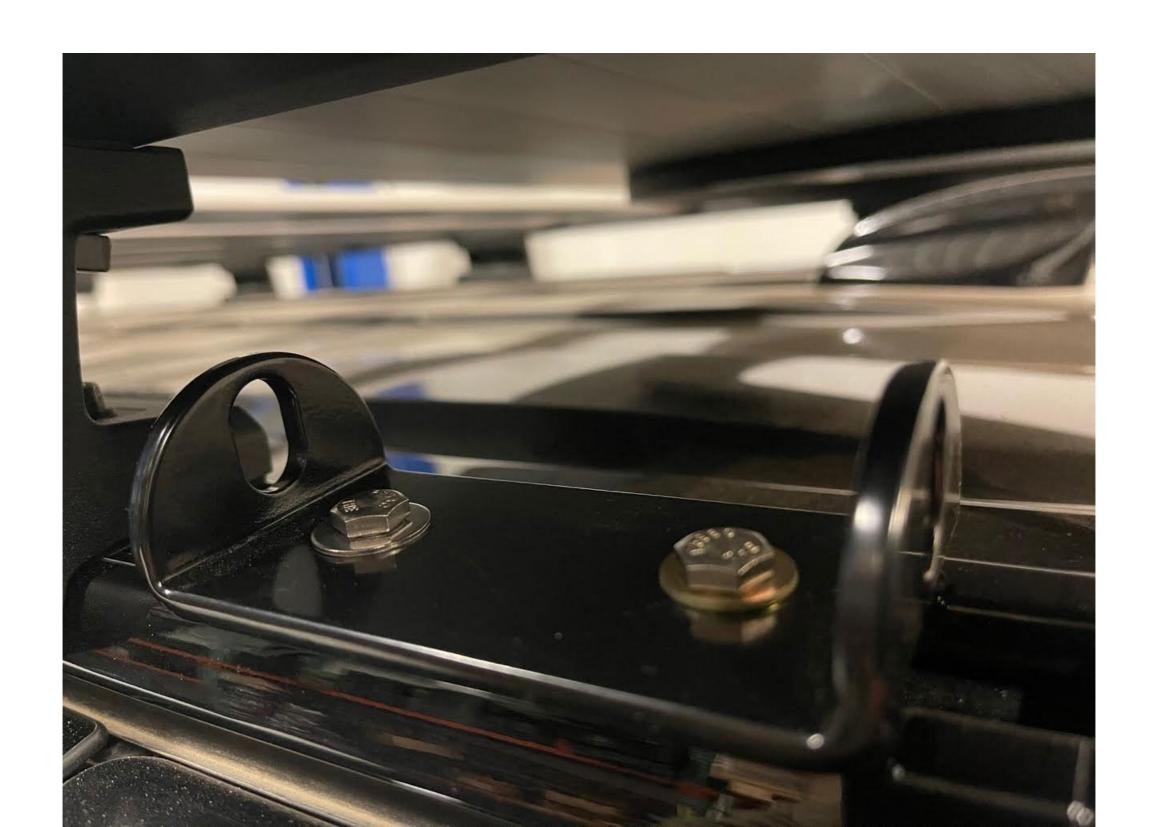
If you have a roof rack you will need to slide the rear mounting bracket out of the way to fit the mounting bolt.
