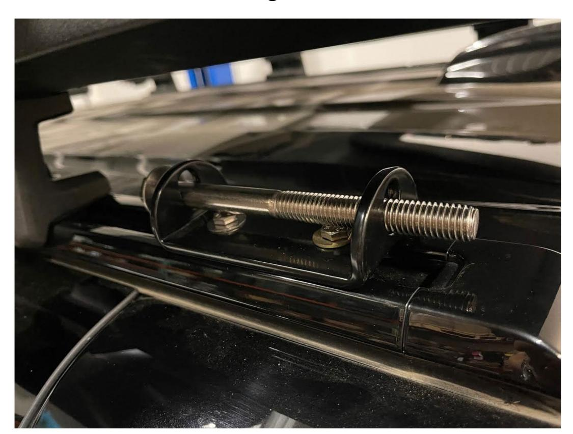
Install the top mount with the hardware in place as shown.
