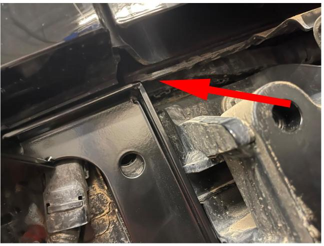
File or grind plastic out of the way if needed.
